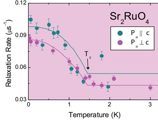
FIGURE A.1: Zero-field relaxation rate in  $\text{Sr}_2\text{RuO}_4$  with the initial muon spin polarization perpendicular and parallel to the  $c$ -axis of the crystal [123].
