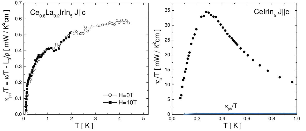
FIGURE C.1: (a) Estimate of inter-plane phonon contribution to the thermal conductivity of  $CeIrIn_5$ . In an impurity-doped sample, where elastic scattering dominates entirely at low temperature, the difference between thermal and electrical conductivities gives the phonon conductivity  $\kappa_{ph}$ . The phonon conductivity is field independent. (b) A comparison between the same phonon contribution and the thermal conductivity of pure  $CeIrIn_5$ .
