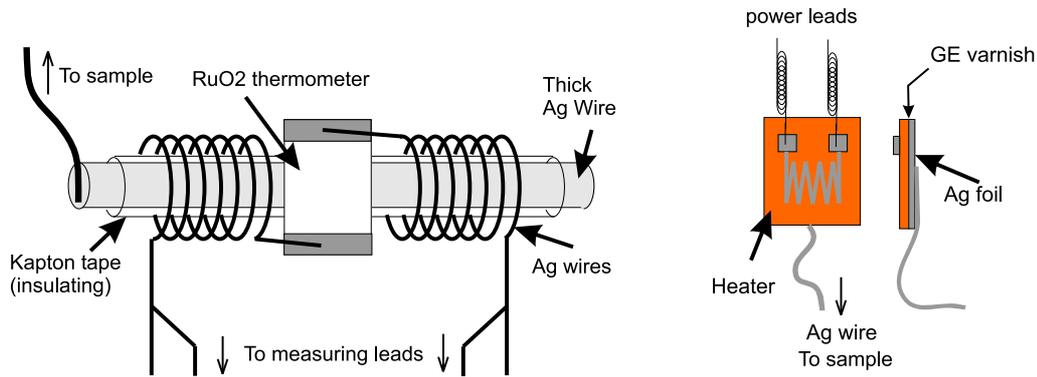
FIGURE 4.2: Schematic of thermometer and heater in our thermal conductivity setup in Dilution refrigerator [162].
