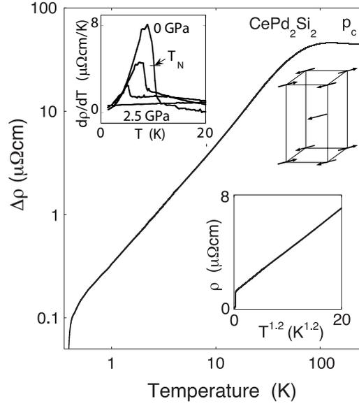
FIGURE 9.10: Temperature dependence of resistivity in  $CePd_2Si_2$  near the critical pressure  $p_c \cong 2.8\text{GPa}$ , where  $T_N \rightarrow 0\text{K}$ . Inset-bottom: resistivity plotted against  $T^{1.2}$ . Inset-top: derivative of electrical resistivity in various pressures [77].
