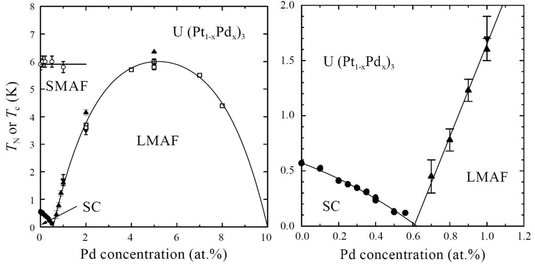
FIGURE 9.11: Magnetic and superconducting phase diagram for  $U(Pt_{1-x}Pd_x)_3$  alloys. SMAF=small-moment antiferromagnetic phase, LMAF=large-moment antiferromagnetic phase, SC=superconducting phase. (Right) The same phase diagram with  $x < 0.012$  (from [50]). Note to the similarity of this figure to Fig. 3.12 for  $CeIr(In_{1-x}Cd_x)_5$ .
