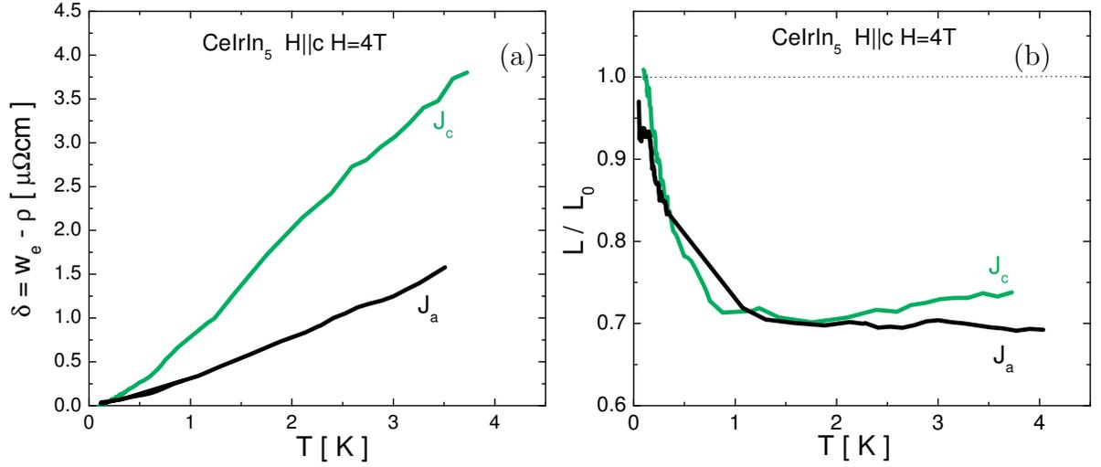
FIGURE 9.6: A comparison between in-plane and inter-plane (a)  $\delta(T) \equiv w_e(T) - \rho(T)$  and (b) normalized Lorenz ratio,  $L/L_0$ , in CeIrIn<sub>5</sub>.
