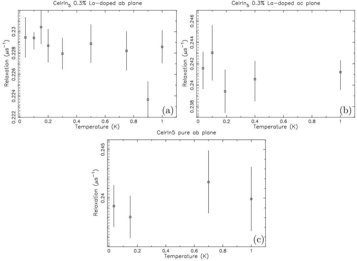
FIGURE A.5: Preliminary analysis of zero field muon spin relaxation rate vs temperature measured in (a)  $ab$ -plane doped, (b)  $ac$ -plane doped and in (c)  $ab$ -plane pure  $\text{CeIrIn}_5$ . It seems there is no enhancement of relaxation rate in the SC state (below  $T_c \approx 0.4$  K).
