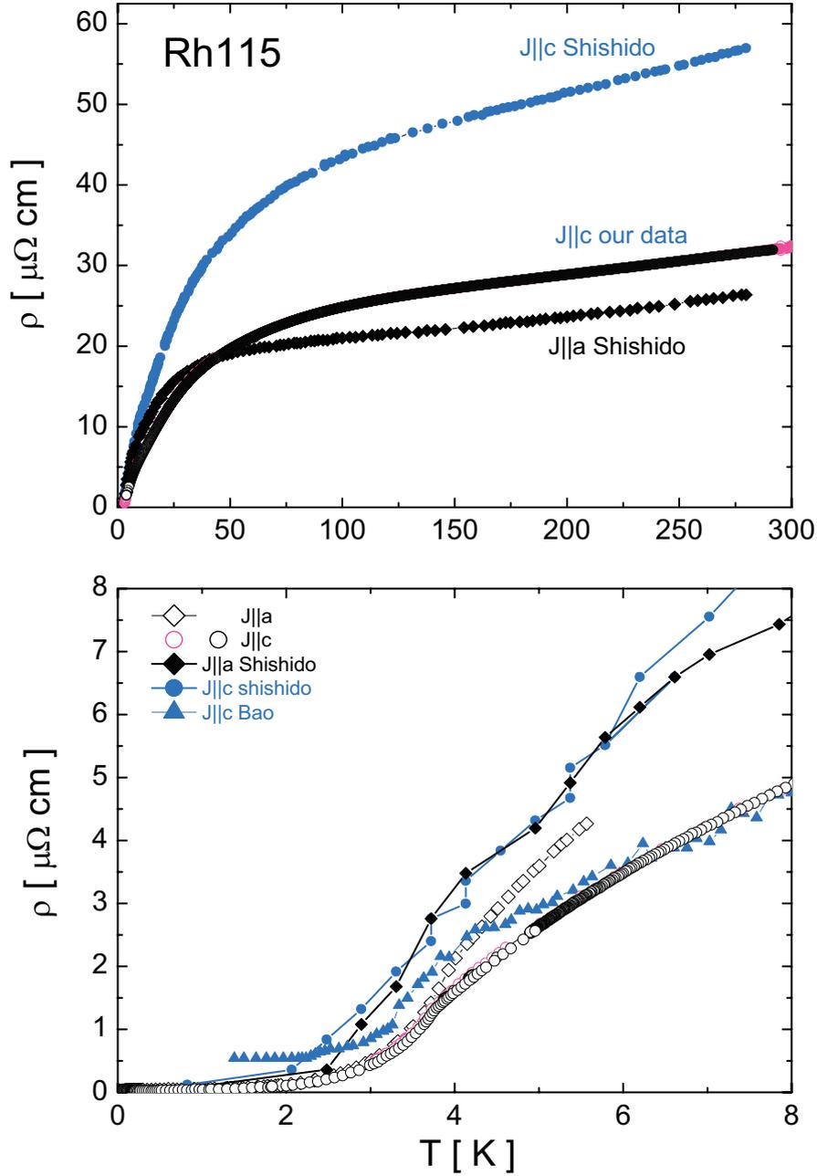
FIGURE B.1: Inter-plane resistivity of  $Rh115$  compared with other group data at high (top) and low temperatures (bottom). Bao data [20] at low temperature seems to behave similar to ours. Note to the same Neel temperature for both current orientations in our measurements (bottom). The electron conductivity is better in the  $c$ -axis than  $a$ -axis direction, consistent with the thermal conductivity results shown later (see Fig. B.3.) (data of other group are taken from [195, 20, 44]).
