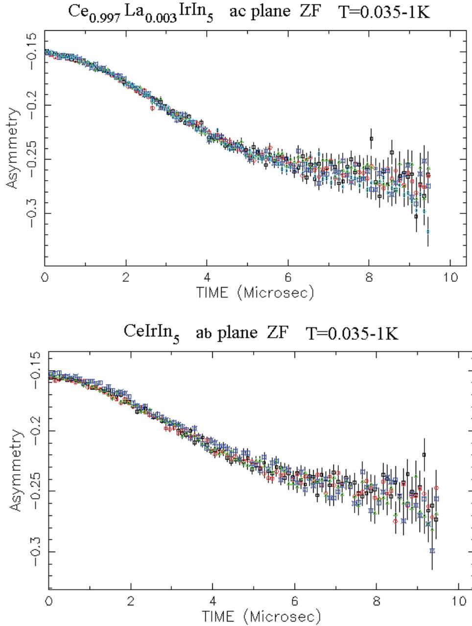
FIGURE A.4: Asymmetry in  $\text{Ce}_{0.997}\text{La}_{0.003}\text{IrIn}_5$  *ac*-plane and pure  $\text{CeIrIn}_5$  *ab*-plane samples at  $T = 35\text{mK}, 100\text{mK}, 150\text{mK}, 200\text{mK}, 300\text{mK}, \dots$  to  $1\text{K}$  (below and above  $T_c$ ). Preliminary analysis of ZF  $\mu\text{SR}$  spectra. All curves have fall on top of each other. The same result was observed for *ab*-plane doped crystals.
