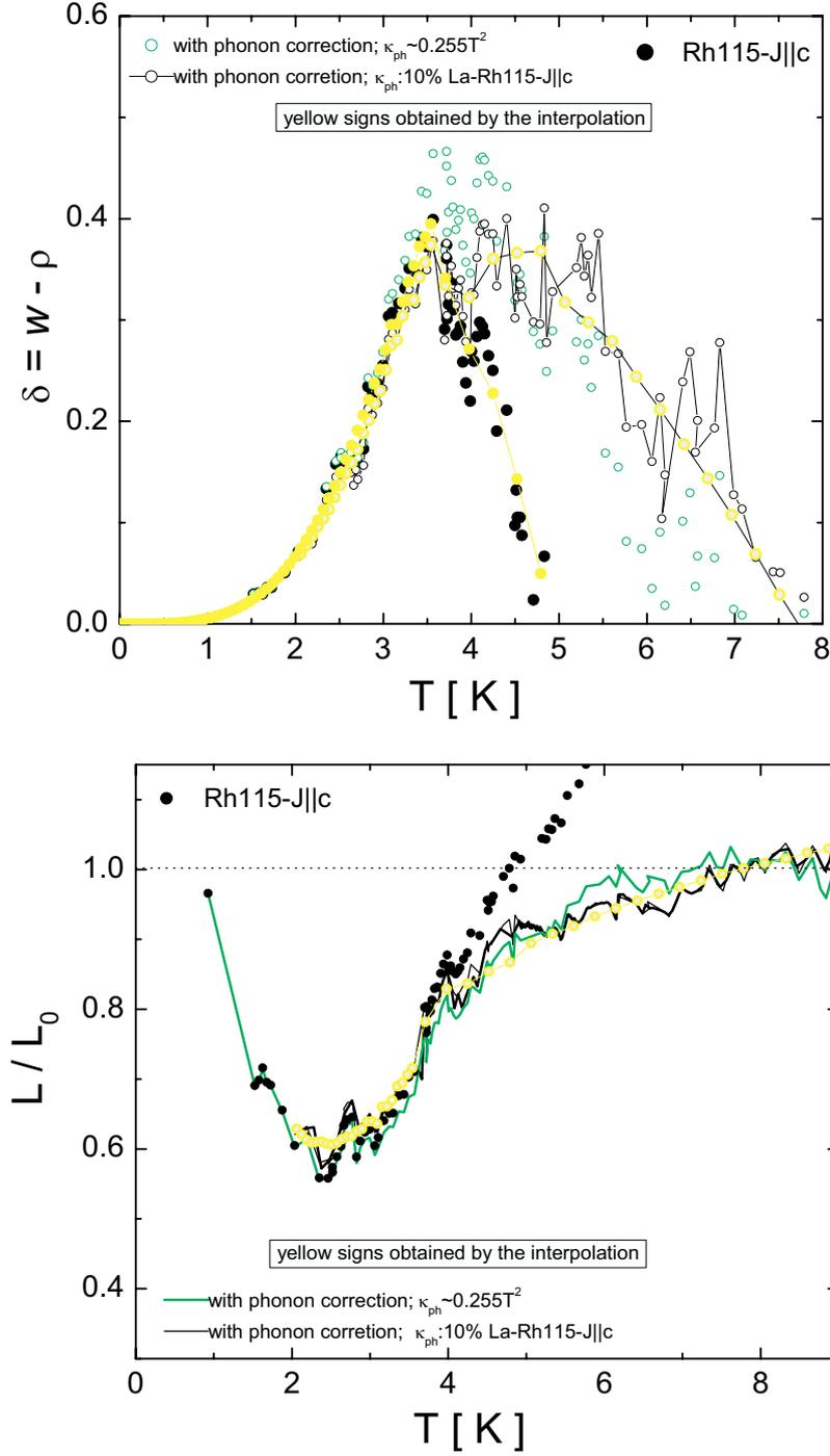
FIGURE B.5: (*Top*) The  $\delta(T) \equiv w_e(T) - \rho(T)$  in the  $c$ -axis  $CeRhIn_5$  vanishes around  $T \cong 8$  K. This is exactly the temperature where the  $\delta$  for  $a$ -axis transport vanishes; see [165]. This can be seen also in the bottom plot, where the  $c$ -axis normalized Lorenz ratio reaches 1 at higher temperature ( $\cong 8$  K). Same notation as Fig. B.3.
