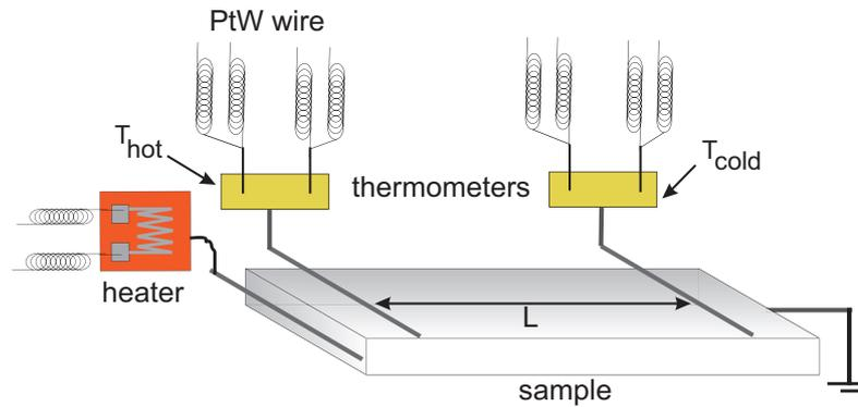
FIGURE 4.1: Schematic of a four-probe thermal conductivity setup (not to scale).
