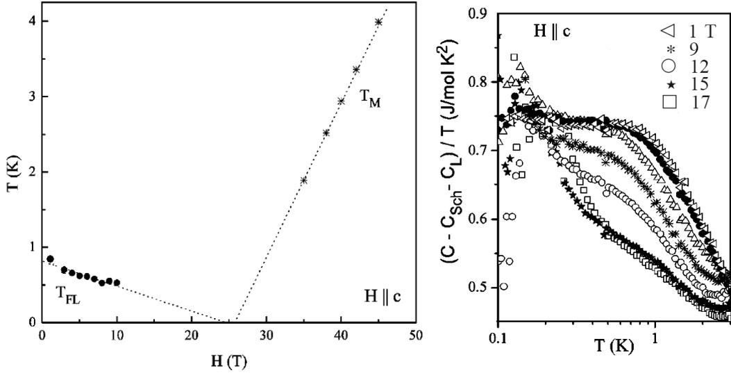
FIGURE 9.9: (Left) The  $H - T$  phase diagram of  $CeIrIn_5$  obtained from specific heat measurement. Fermi-liquid temperatures  $T_{FL}$  derived from the electronic specific heat.  $T_M$  is the metamagnetic transition temperature taken from [108]. (Right) Electronic specific heat, obtained by subtracting the Schottky and lattice contributions from the total specific heat, as a function of temperature at various magnetic fields up to 17 T. Fig adapted from [38].
