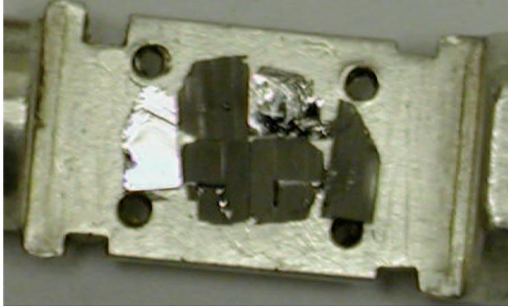
FIGURE A.3: Sample mount for zero field  $\mu$ SR measurements. The probe is inserted such that the initial muon spin polarization is  $\perp$  to the face of the crystals.
