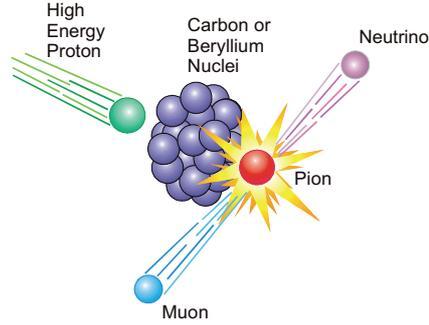
FIGURE A.2: A schematic of producing muon beams, using high-energy protons to produce short-lived muons.
