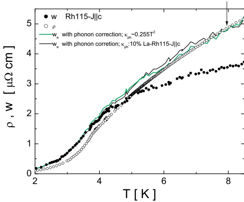
FIGURE B.4: Electrical resistivity ( $\rho$ ) compared to thermal resistivity ( $w$ ) in Rh115 ( $J||c$ ). Solid lines show the electronic thermal resistivity ( $w_e$ ); see notation in Fig. B.3. The electrical resistivity and the electronic thermal resistivity meet each other around  $T = 8K$ .
