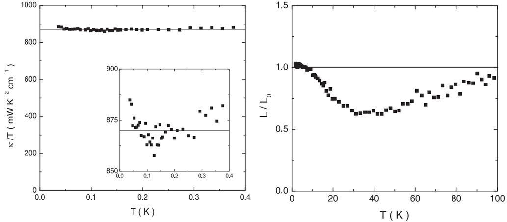
FIGURE 4.3: Test experiment of the thermal conductivity setup on pure silver wire. Inset shows the 3% scattering in the data, confirming the high precision of the thermal conductivity mount [36].
