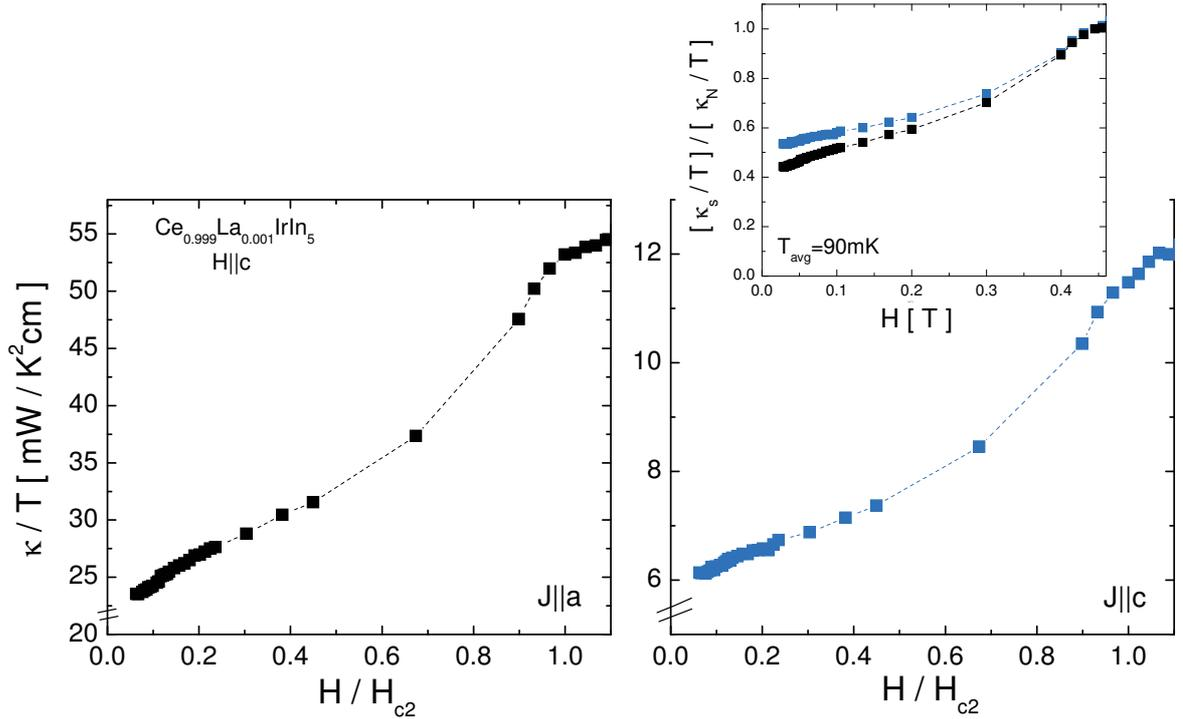
FIGURE D.1: The in-plane and inter-plane thermal conductivity,  $\kappa/T$ , of 0.1% La-doped  $CeIrIn_5$  at  $T = 90$  mK as a function of applied field. Note to the similar behaviour of two heat current directions. We argue impurities broaden the linear point nodes at the poles so that they behave as a line node.
